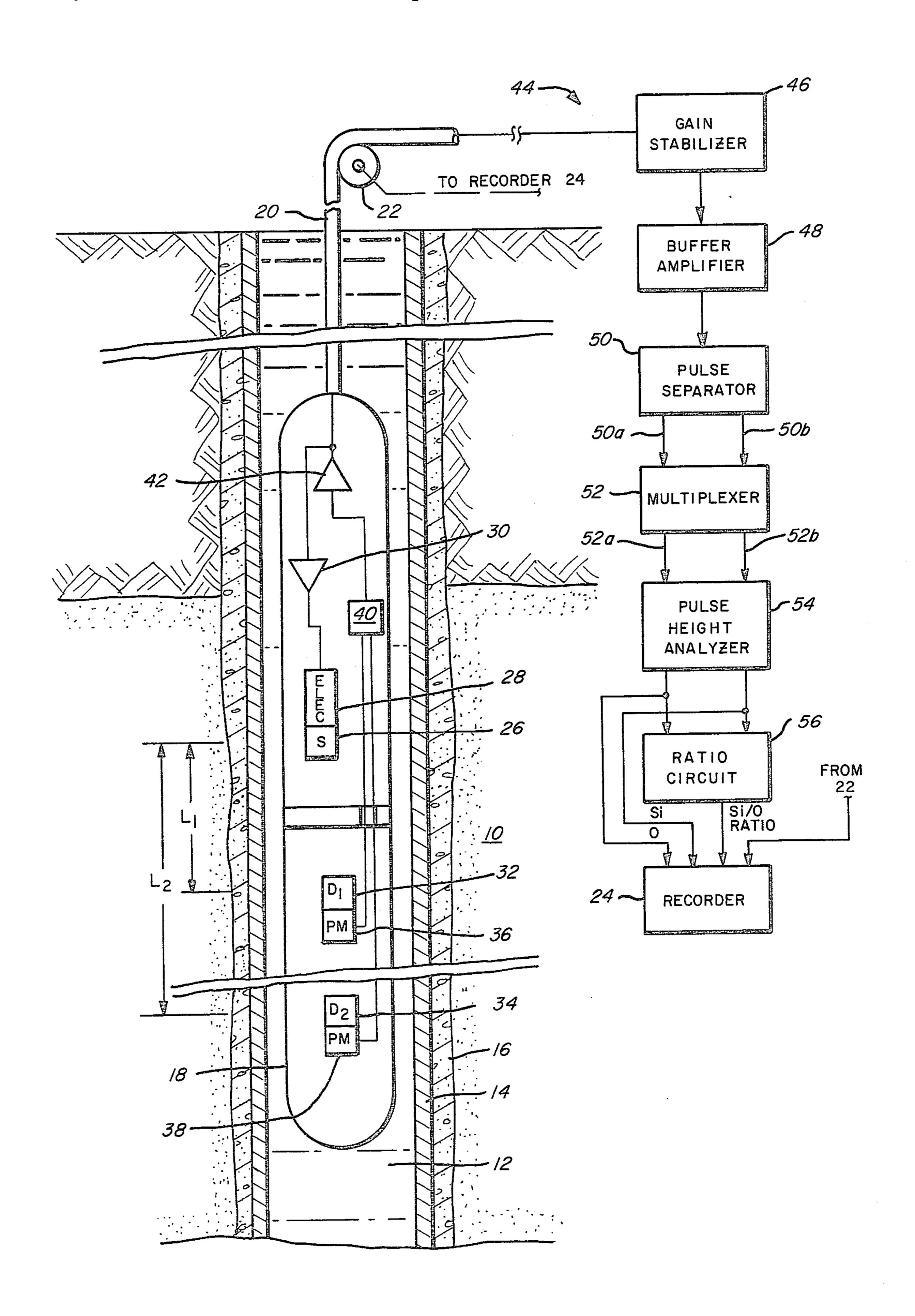
NUCLEAR WELL LOGGING WITH NEUTRON SOURCE AND SEPARATE SPACED RADIATION DETECTORS TO DETERMINE SILICON/OXYGEN RATIO
