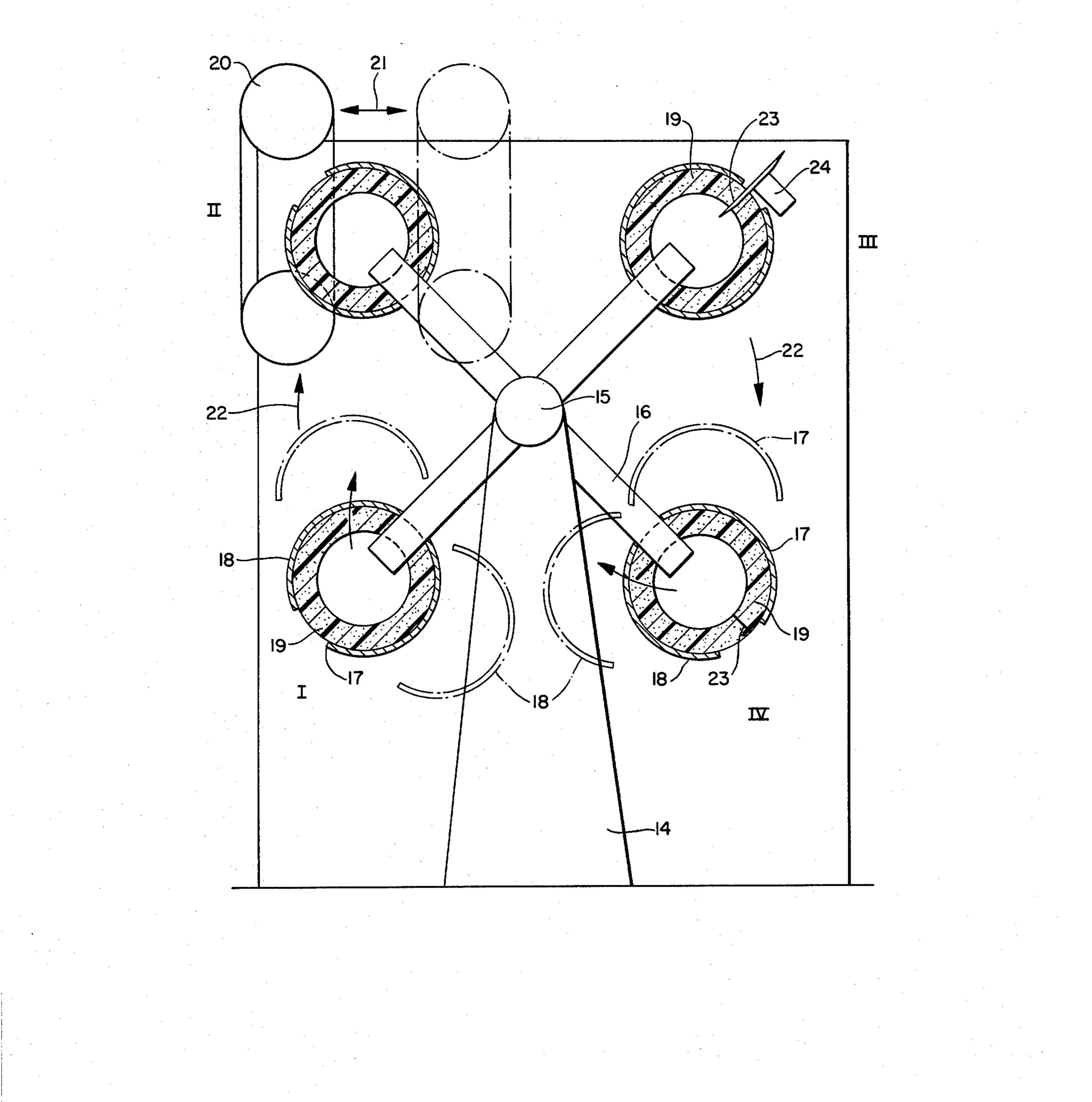
The invention relates to a machine installation or arrangement for the production of thick-walled insulating pipes formed of elastic, laminatable foamed synthetic resin sheets as well as a process for forming such pipes.
