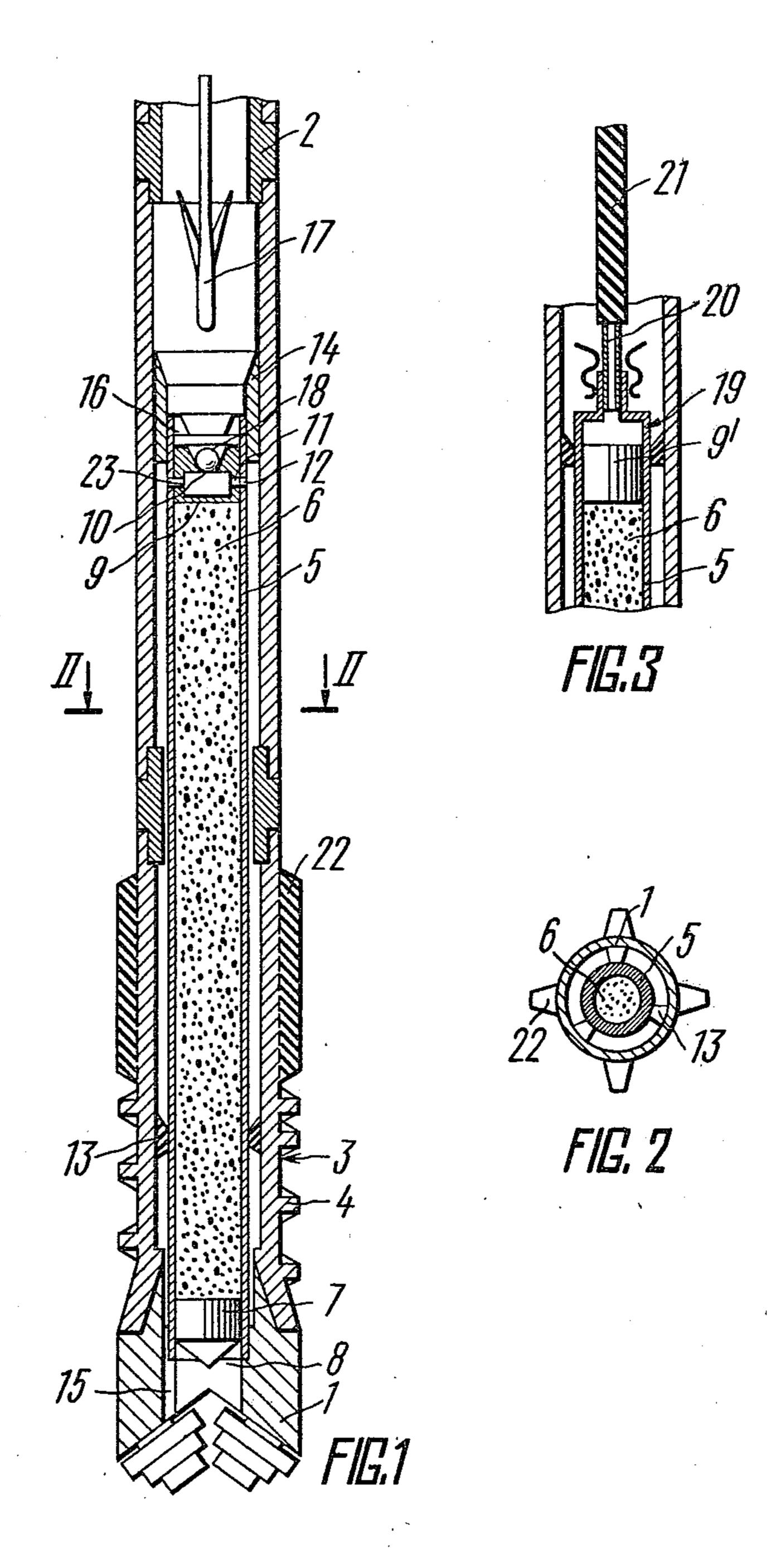
ARRANGEMENT FOR FULL HOLE DRILLING
