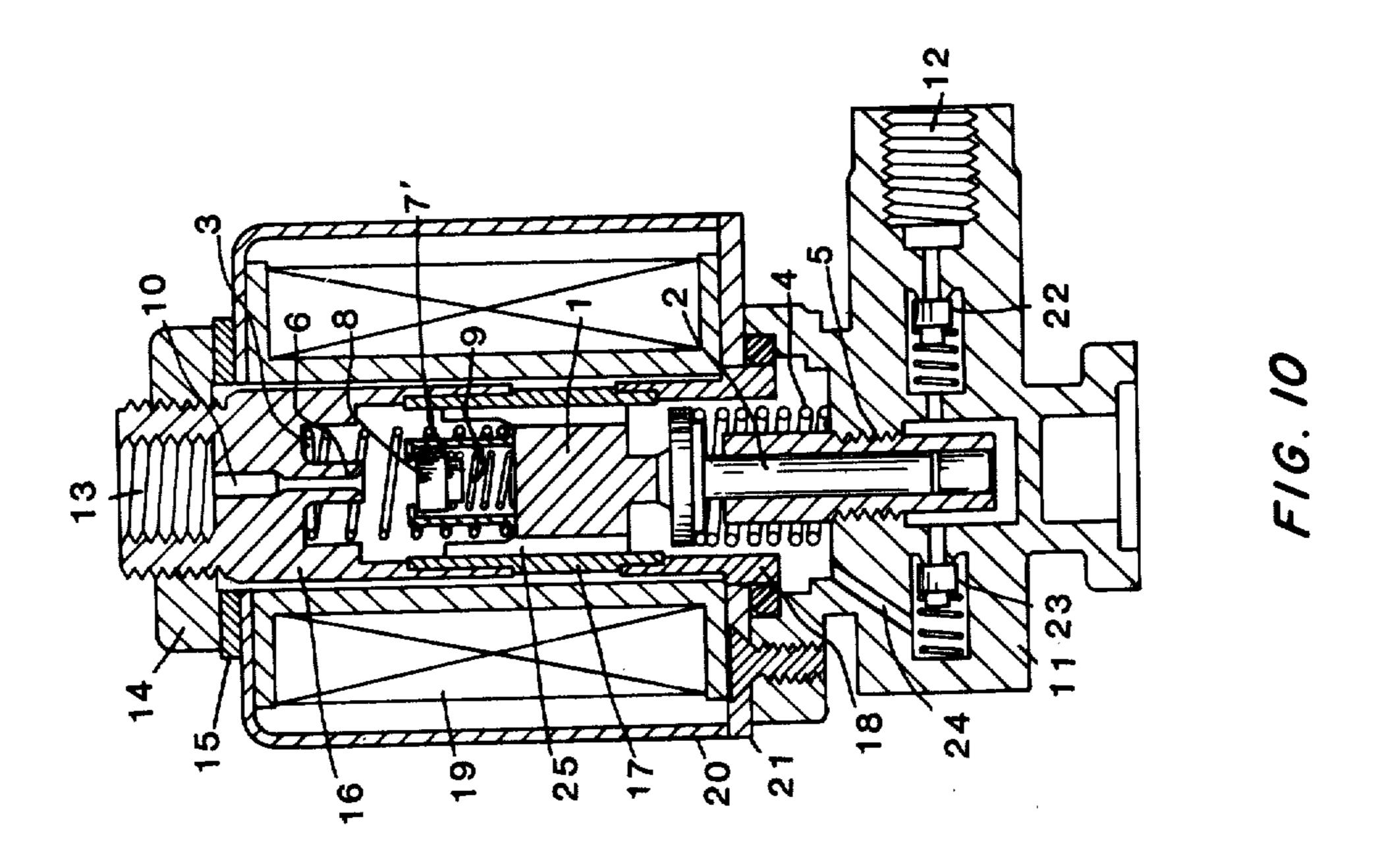
The valve body engages a valve seat in a discharge passage to close the discharge passage during a pump shut-down. The valve body is liberated from the valve seat to open the discharge passage during pump operation
