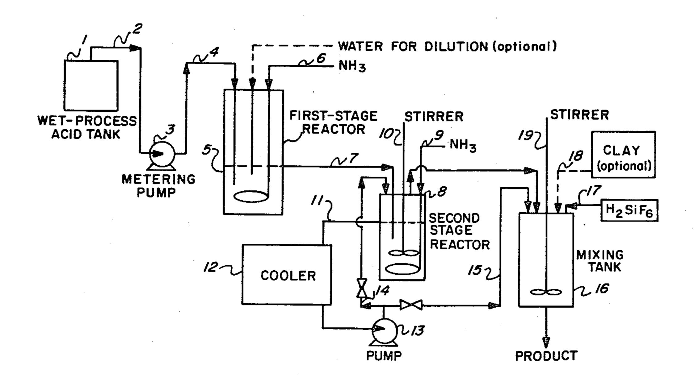
PRODUCTION OF AMMONIUM PHOSPHATE SUSPENSION FERTILIZERS BY
