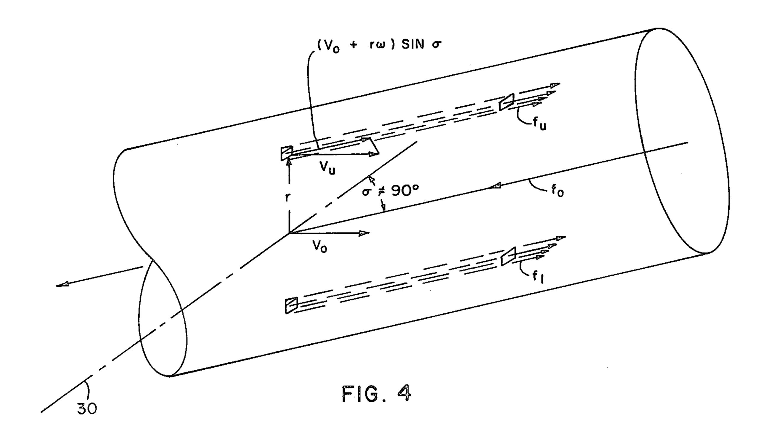
FIGS. 3 and 4 are geometry schematics for indicating the laser aspect angle to the reflectors.
