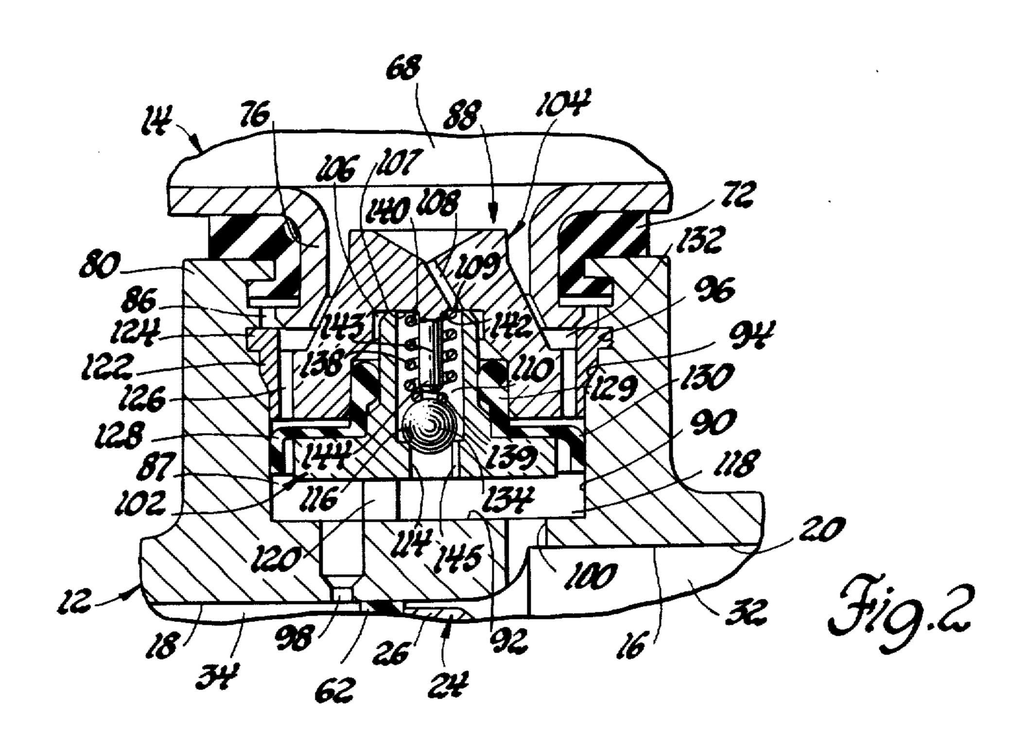
radially outward of the spring seat area so that fluid flow occurs predominantly outside the coils of the spring, and need not pass between the coils. This eliminates fluid flow noise which occurs as flow passes between closely positioned spring coils.
