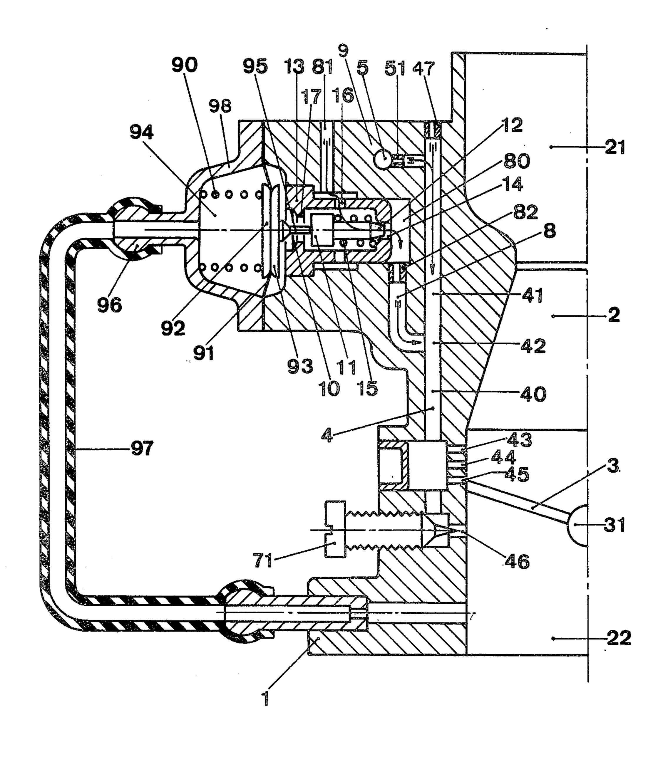
DEVICE ADAPTED TO CORRECT THE AIR-FUEL RATIO OF THE MIXTURE DELIVERED BY A CARBURETOR DURING THE PERIODS OF OPERATION AT LOW LOADS OF A MOTOR VEHICLE ENGINE
