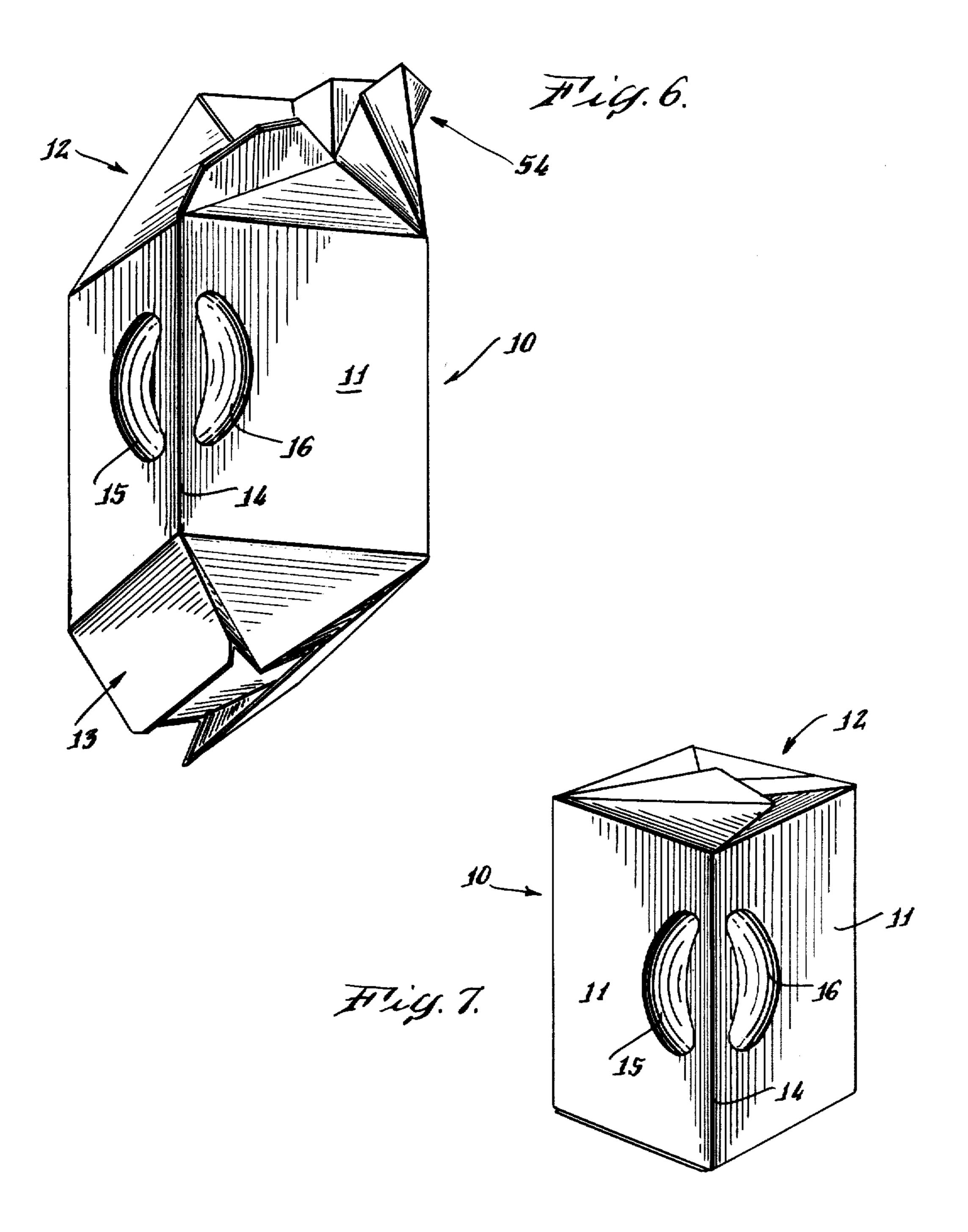
METHOD AND APPARATUS FOR FORMING A PLASTIC FLUID CONTAINER WITH AN INTEGRAL HANDLE
