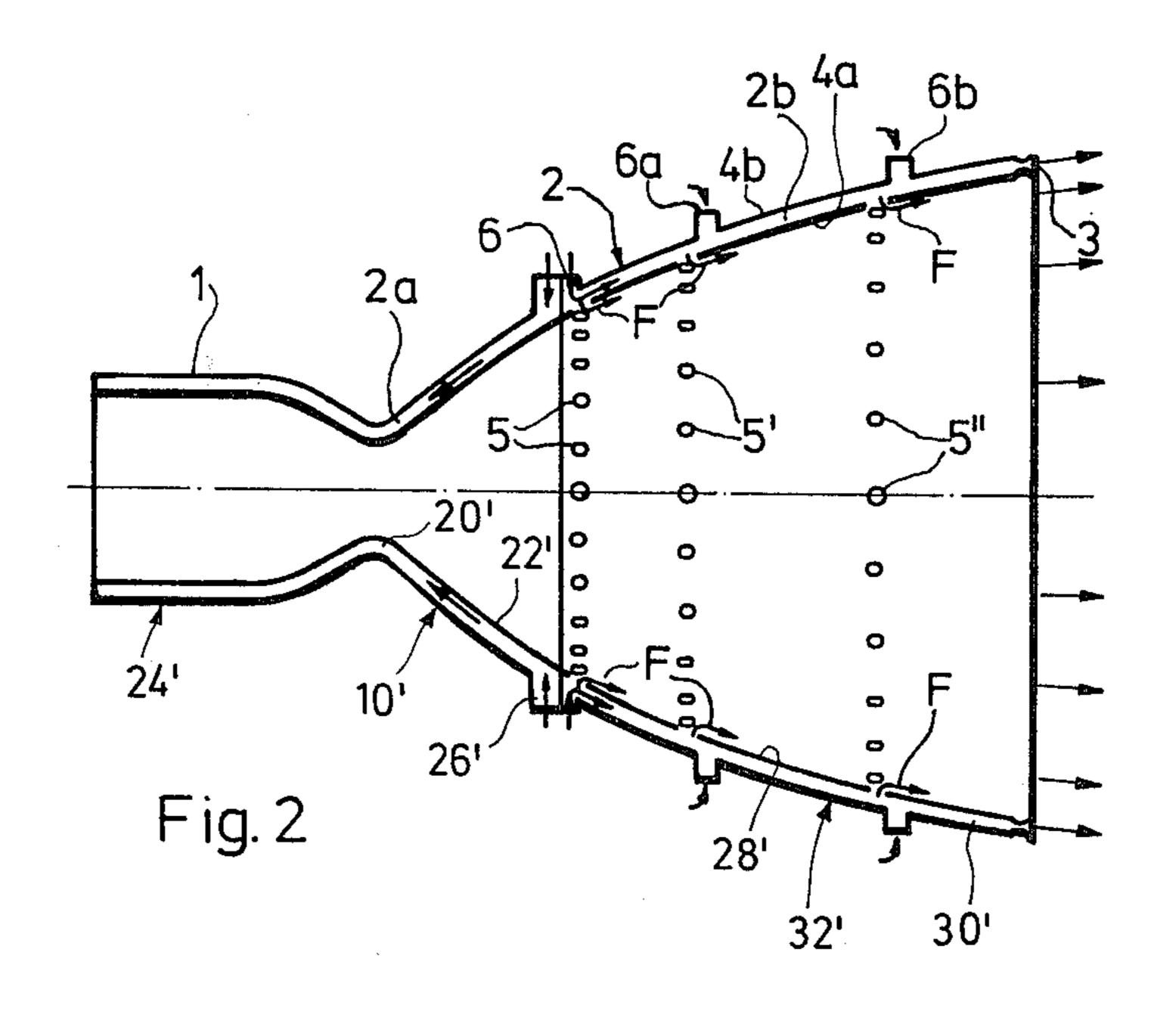
ity inside the cooling channels due to the occurring high pressure losses and the attainment of the speed of sound.
