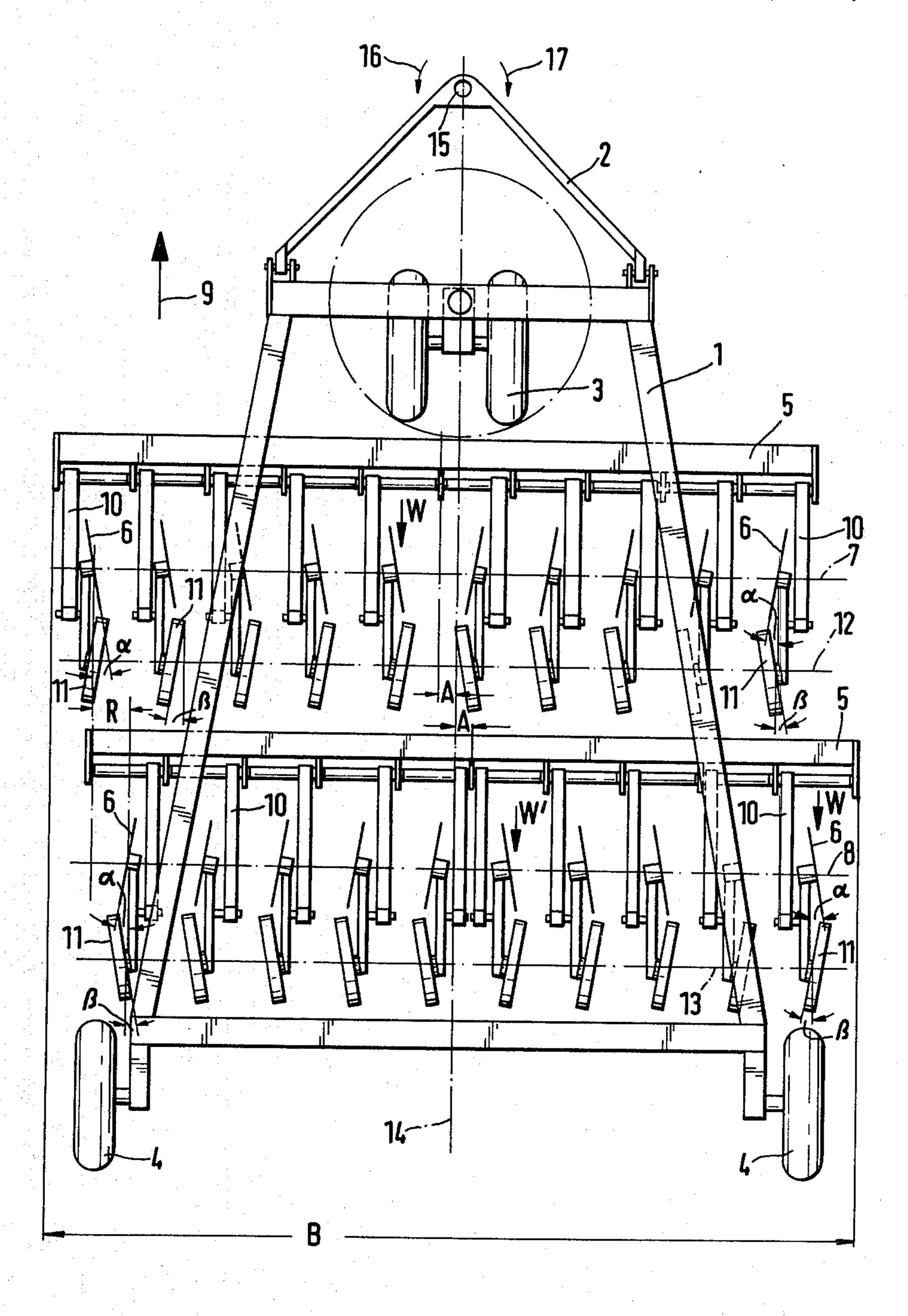
The invention relates to a seed drill having a frame on which single-disk furrow openers set at an acute angle to the direction of travel are arranged by means of mounts, for displacement in the vertical plane, in an alternating and staggered pattern in two rows disposed one behind the other.
