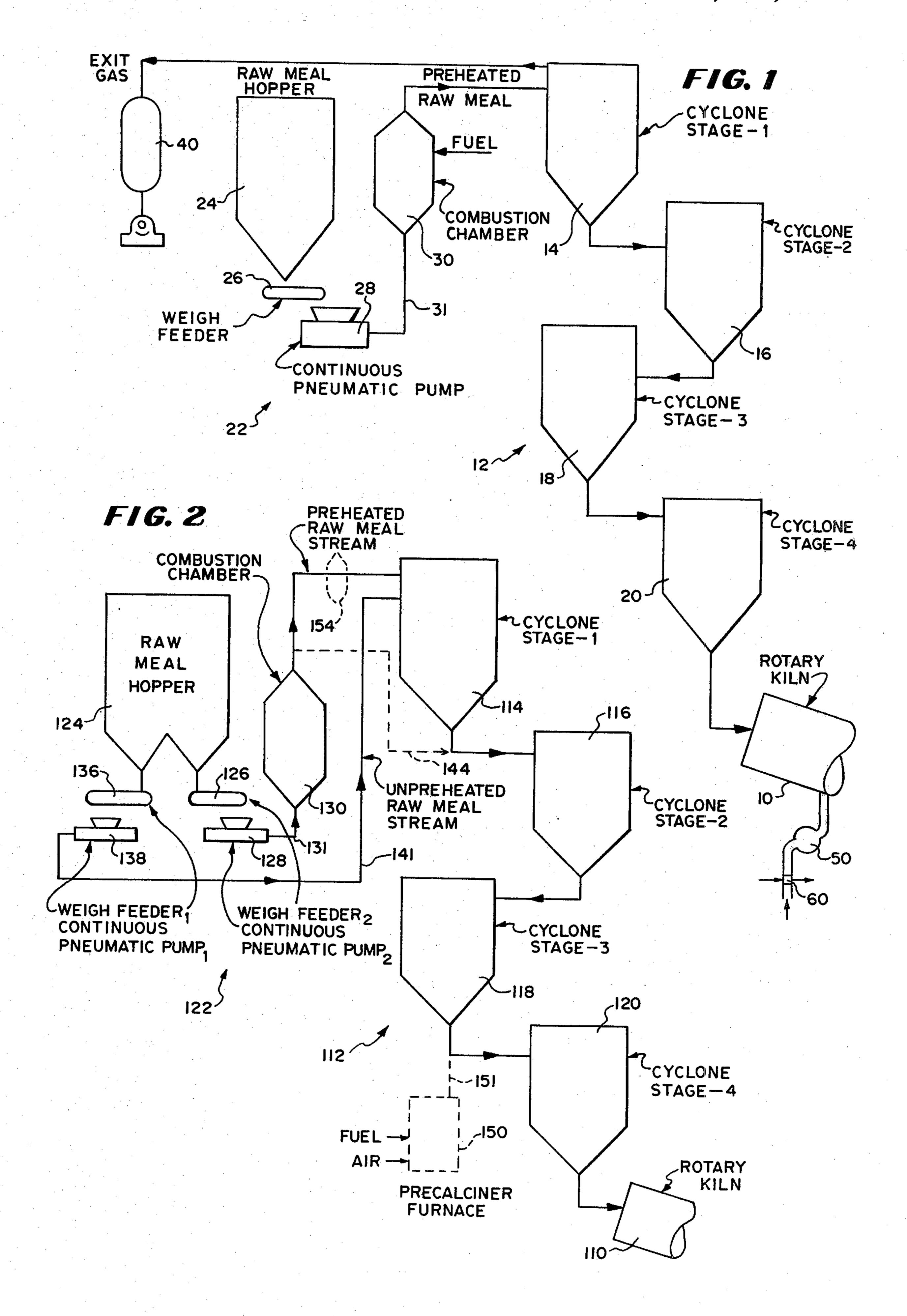
METHOD AND APPARATUS FOR PREHEATING DRY RAW MEAL PRIOR TO INTRODUCTION OF THE MEAL INTO A SUSPENSION CYCLONE PREHEATER SYSTEM SUPPLYING A ROTARY KILN
