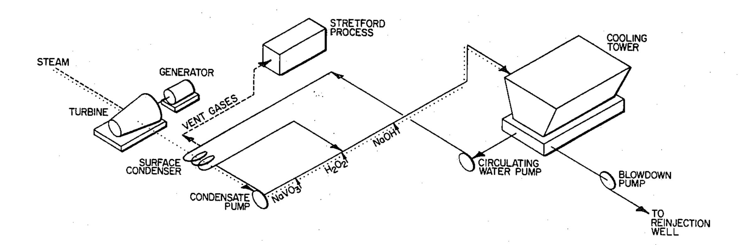
GEOTHERMAL POWER PLANT SURFACE CONDENSER TYPE
