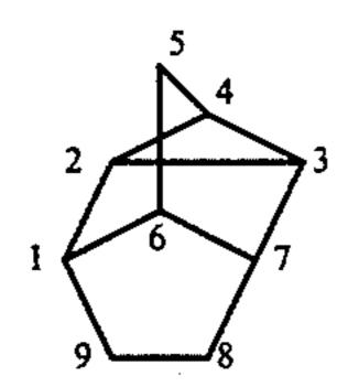
A substituent at the 8-position which lies above the 30 plane formed by carbon atoms 1,6,7,8 and 9 is defined as having the exo-configuration. A substituent at the 8-position which lies below this plane is defined as having the endo-configuration.
