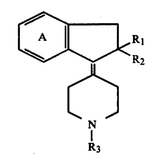
wherein R<sub>1</sub> and R<sub>2</sub> are alkyl, R<sub>3</sub> is hydrogen, alkyl, alkenyl, phenylalkyl or a group —(CH<sub>2</sub>—CH<sub>2</sub>—O)- $_n$ —R<sub>4</sub> in which n is 1 to 3 and R<sub>4</sub> is hydrogen or an acid residue, and the ring A is unsubstituted or substituted, with the proviso that when R<sub>3</sub> is methyl the ring A is substituted. The compounds are useful in the treatment and prophylaxis of allergic conditions.
