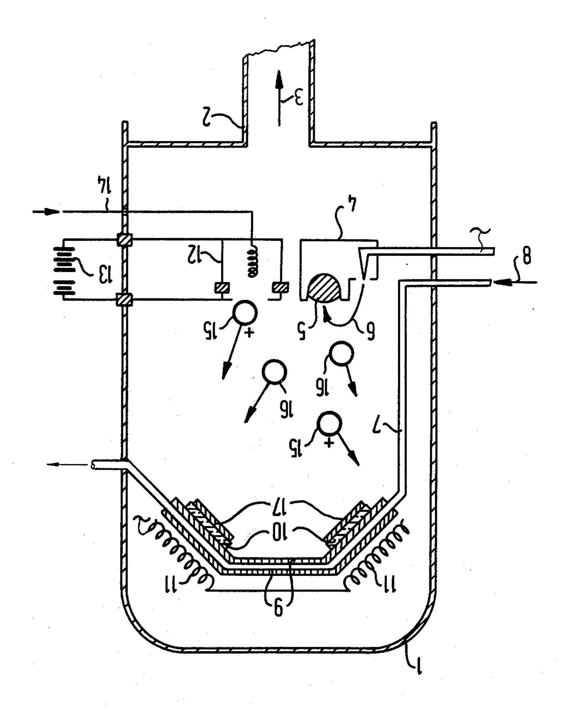
METHOD OF PRODUCING LOW-RESISTANT, MONOCRYSTALLINE METALLIC LAYERS BY IMPLANTING IONS INTO A POLYCRYSTALLINE METAL LAYER AND HEATING TO PRODUCE A MONOCRYSTALLINE LAYER
