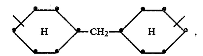
in which the rings can be substituted by  $C_1$ – $C_4$ -alkyl; a preferred meaning is 1,4-cyclohexylene. An aromatic radical G can be  $C_6$ – $C_{10}$ -arylene, such as 1,3- or 1,4-phenylene or 1,5-naphthylene, or a bicyclic radical of the formula
