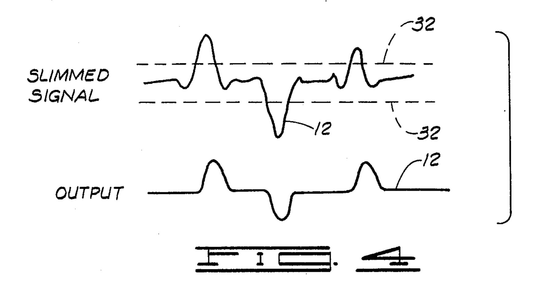
FIG. 4—illustrates the slimmed signal and the output of the slimmed signal from the base line clipper with variable threshold.
