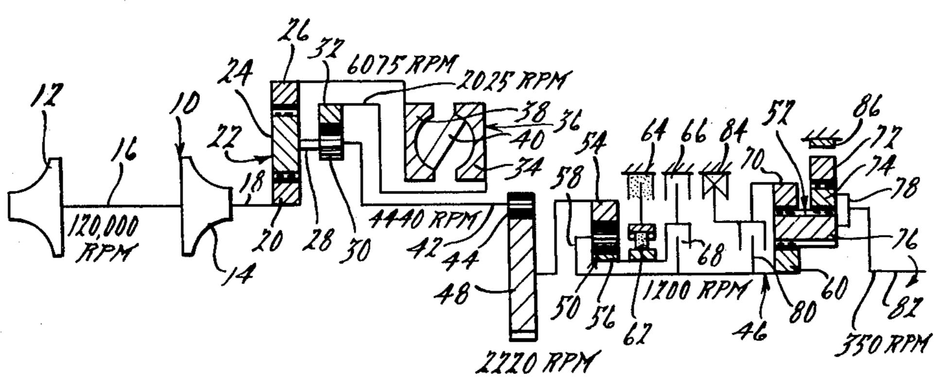
First Ratio-No Engine Braking
