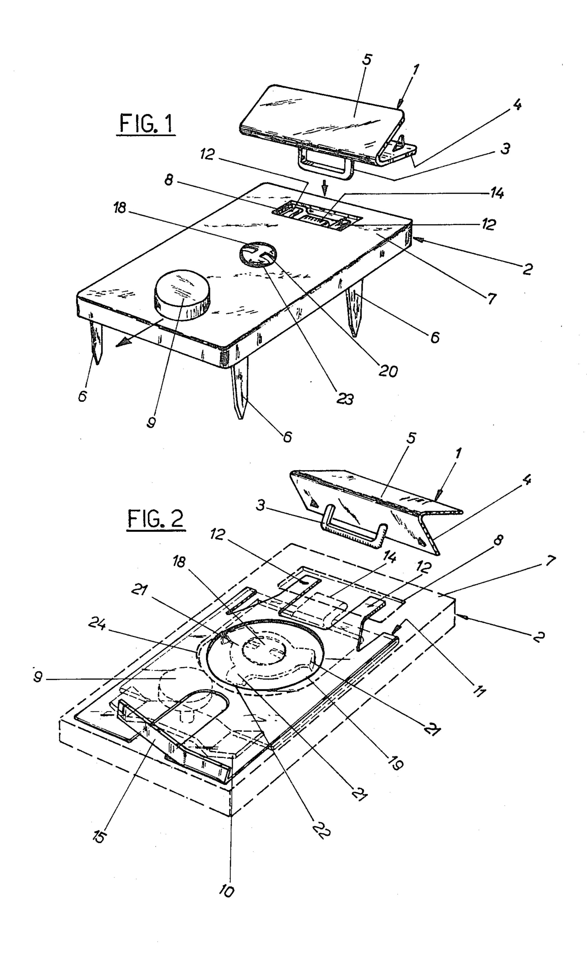
LOCK WITH A RESILIENT ELEMENT ACTING BOTH AS THE EJECTOR AND AS THE SLIDER RETURN SPRING, FOR BAGS, BRIEF-CASES, SHOULDER BAGS AND THE LIKE
