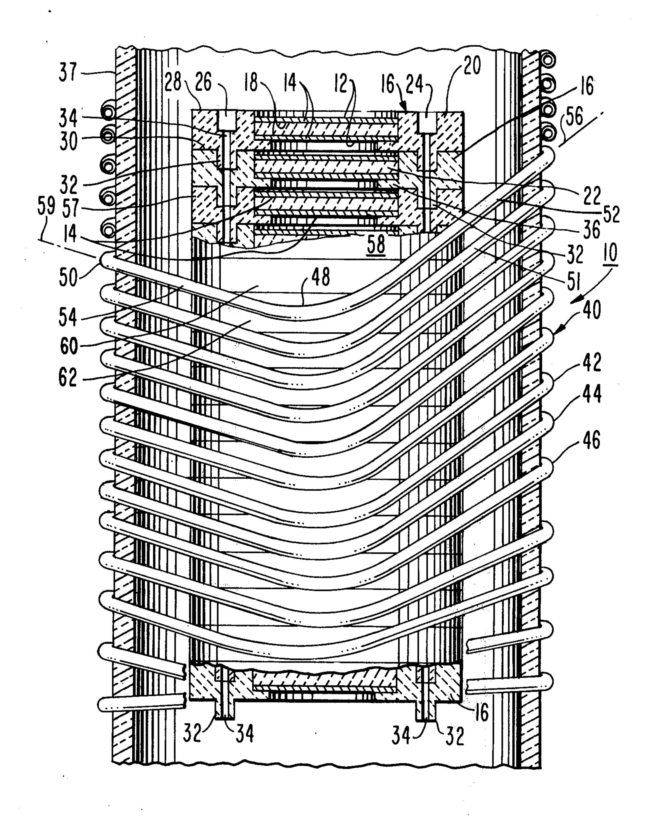
RF HEATING COIL CONSTRUCTION FOR STACK OF SUSCEPTORS
