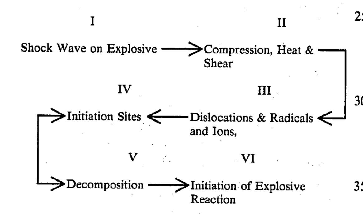
In the first step (I) a shock wave is applied to the explosive either by a mechanical, vibrational, thermal or electric shock. The non-explosive getter additive of 40 the present invention can increase the amount of shock necessary to initiate the explosion. This is important in formulating explosives since it allows the use of more powerful explosives in conventional applications where the explosives were previously too sensitive.
