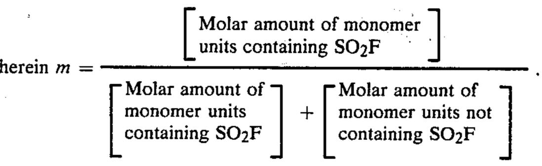
This substantially corresponds to the situation that the equivalent weight of the copolymer is usually in the range of from 1,000 to 2,800, preferably in the range of from 1,100 to 2,000, more preferably in the range of from 1,100 to 1,700.
