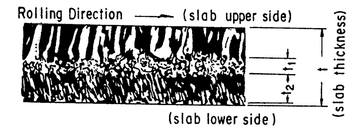
METHOD FOR HEATING CONTINUOUSLY CAST STEEL SLAB FOR PRODUCTION OF GRAIN-ORIENTED SILICON STEEL SHEET HAVING HIGH MAGNETIC FLUX DENSITY
