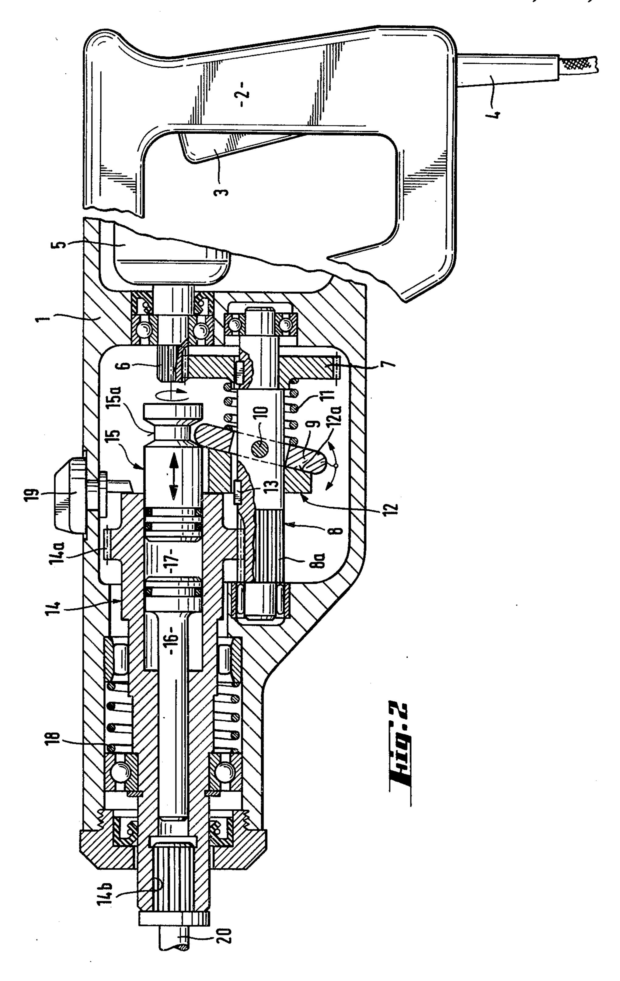
HAMMER DRILL OR CHIPPING HAMMER DEVICE
