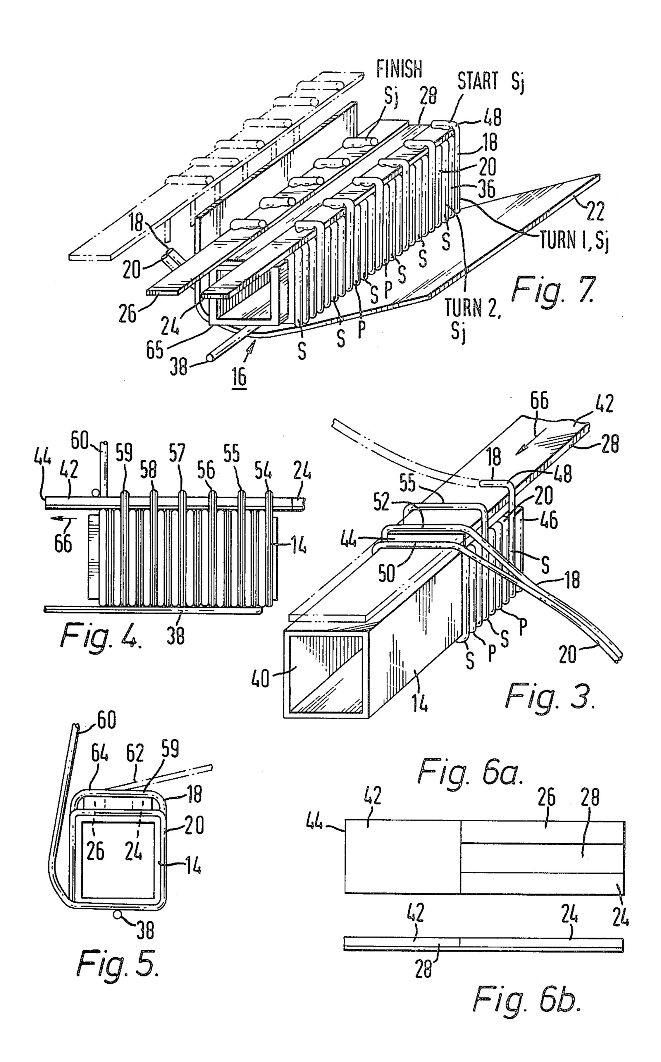
winding a primary coil and then winding the secondary coils about the primary coil or vice versa, also reduce the coupling coefficient.
