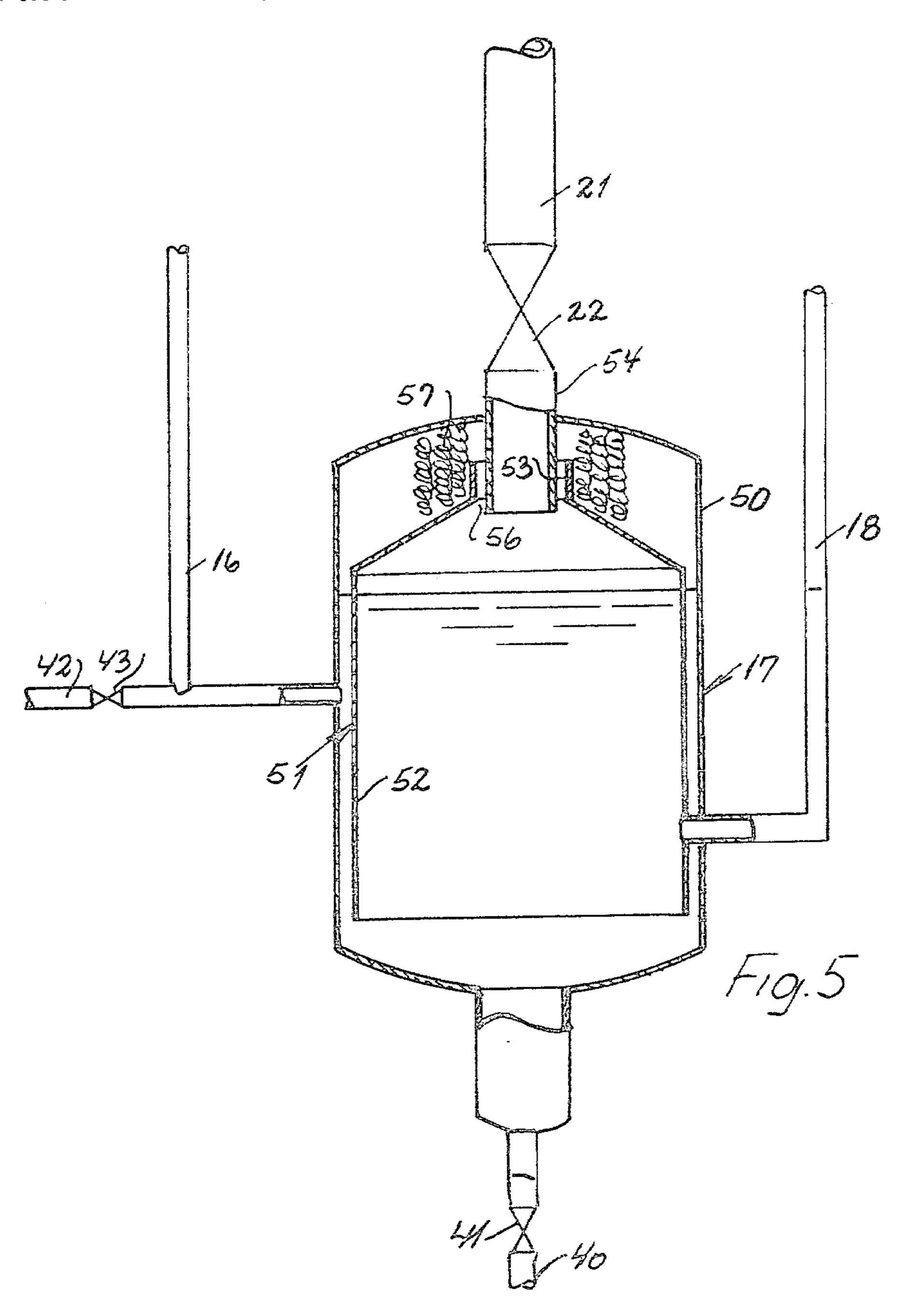
FREEZING OR COOLING PLANT COMPRISING AN OIL SEPARATOR
