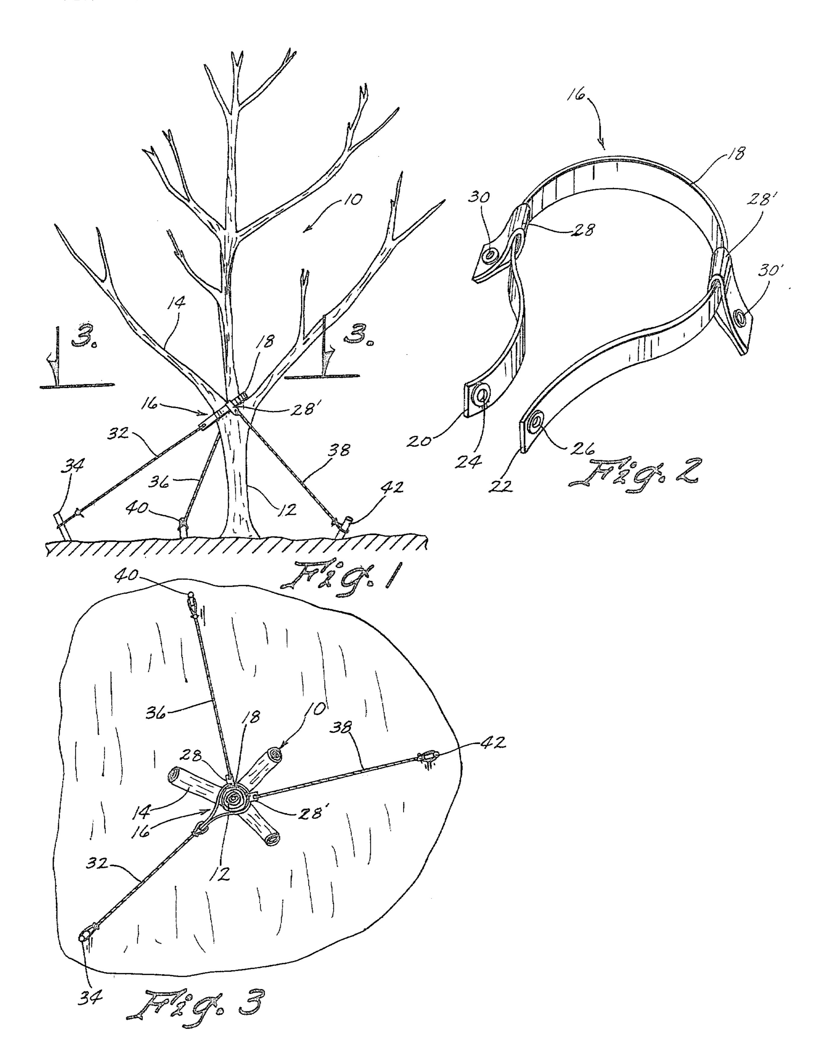
MEANS FOR SECURING A TREE TO GROUND STAKES
