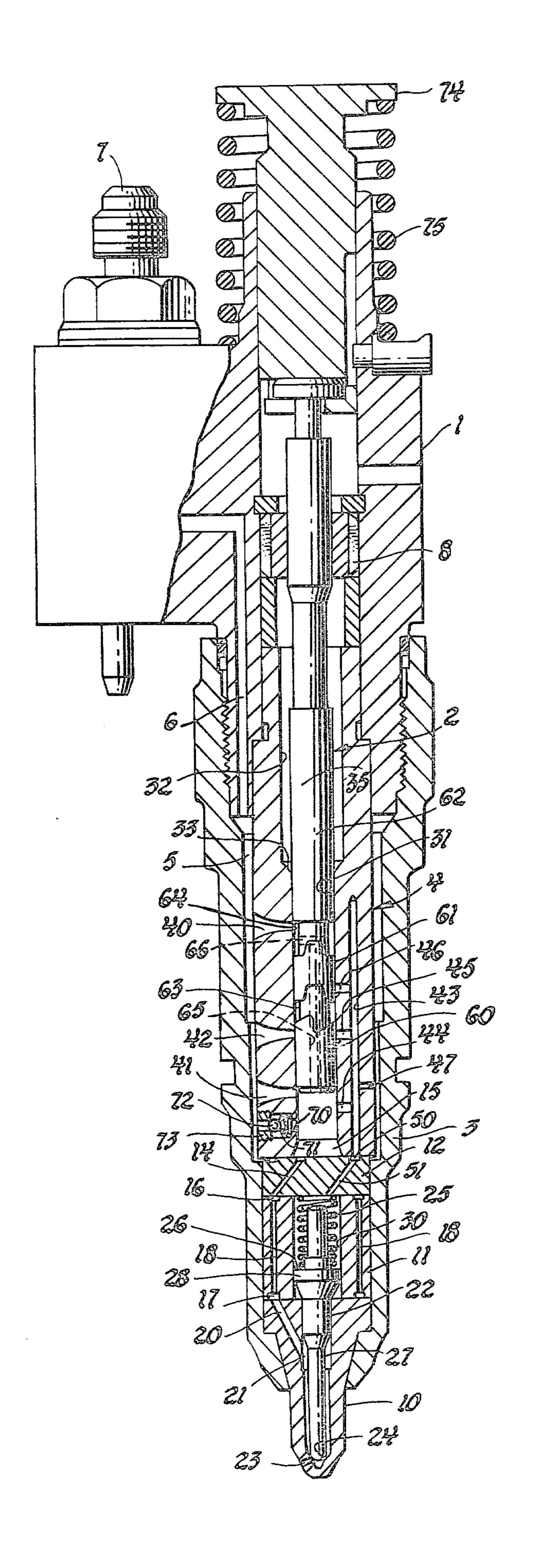
injection timing via the hydraulic needle valve of the injector.
