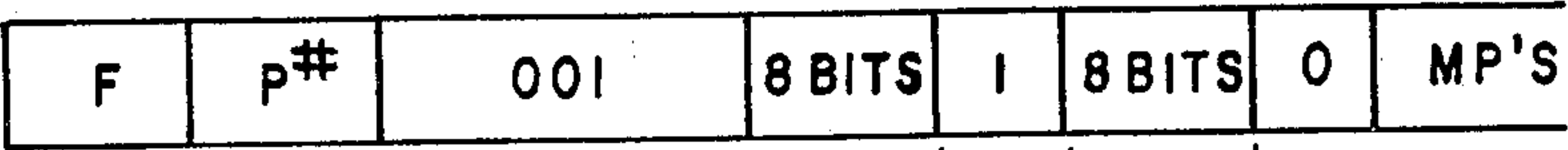
Fig. 10 1st ADDRESS 2nd ADDRESS HEADER FOR SYNCHRONOUS MULTI-USER PACKET
