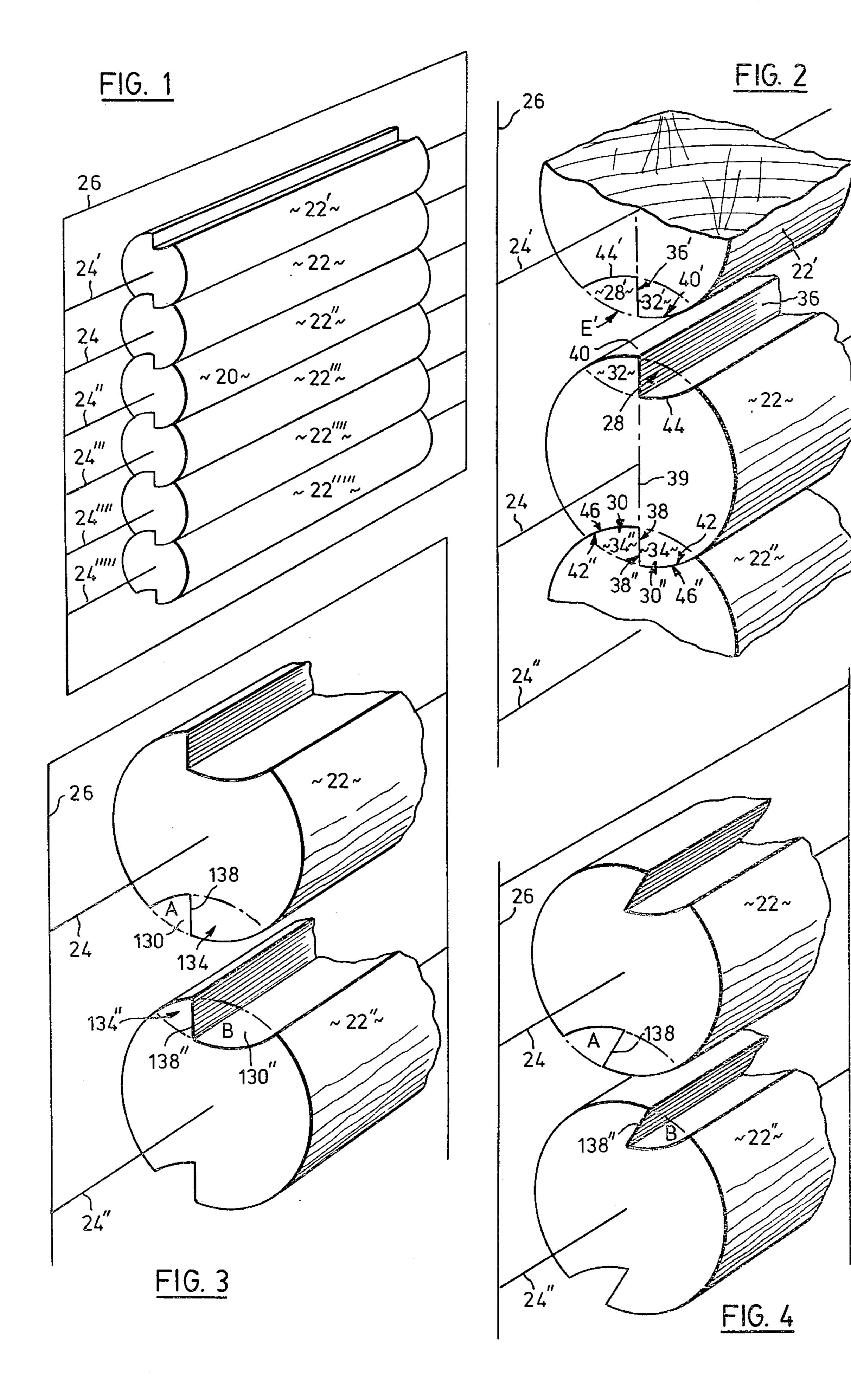
This invention relates to an elongate structural member shaped for use with other such members in the construction of walls or similar structures formed by interfitting the members side by side.
