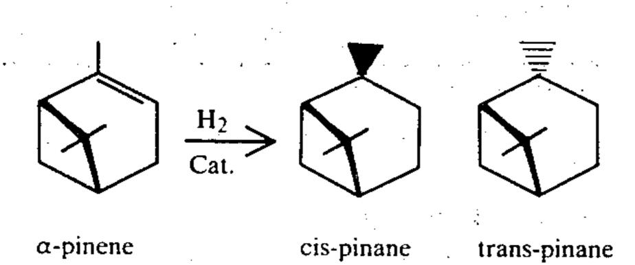
Advantageously, the hydrogenation is carried out under conditions which favor formation of the cis-iso- 55 mer of pinane over the trans-isomer. Factors influencing or promoting such stereoselectivity include, for example, the hydrogenation catalyst and the hydrogenation pressure, temperature and reaction time. In general, lower temperatures, higher pressures and longer 60 reaction times favor production of cis-pinane from  $\alpha$ -pinene.
