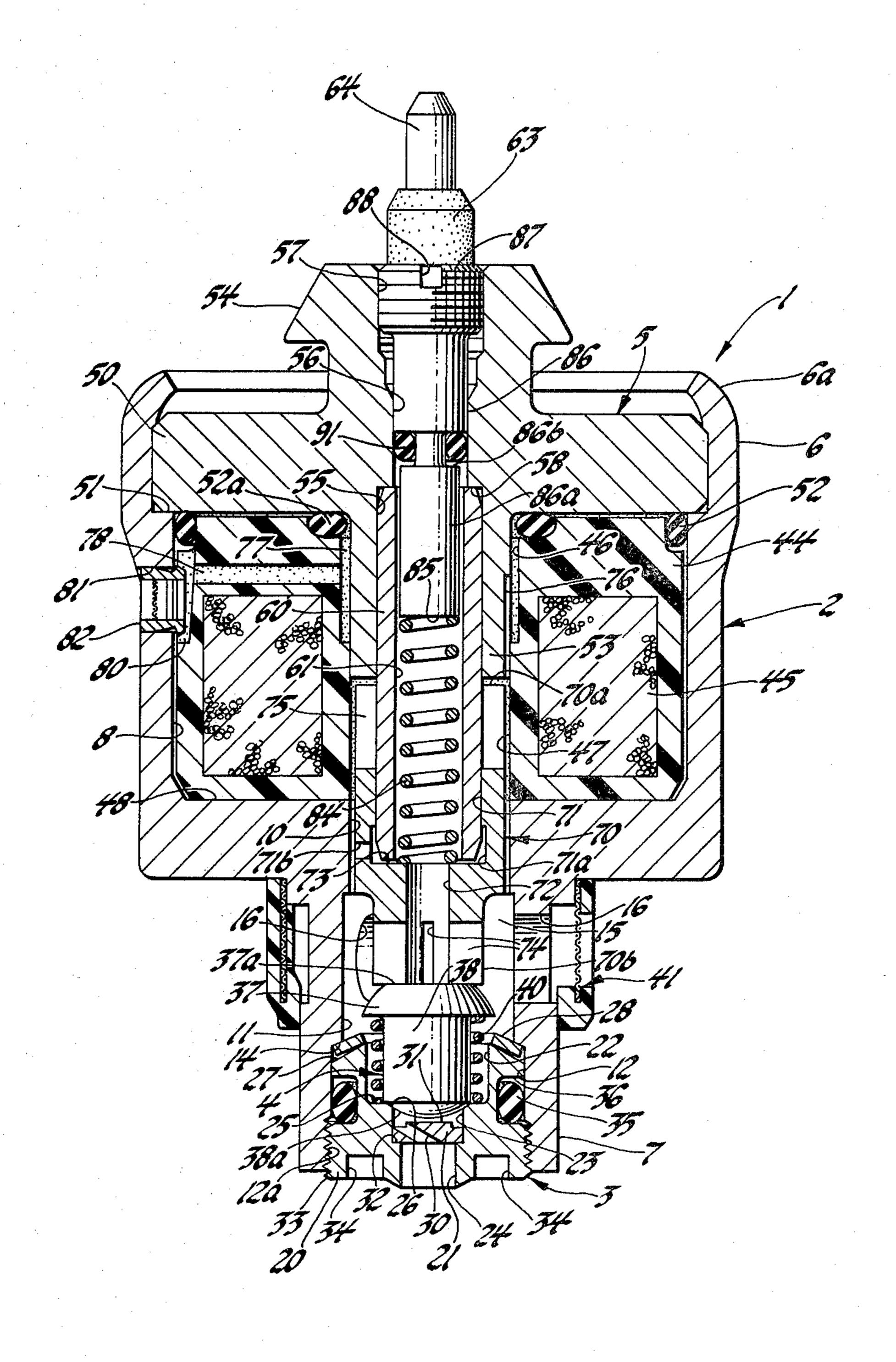
ELECTROMAGNETIC FUEL INJECTOR WITH
