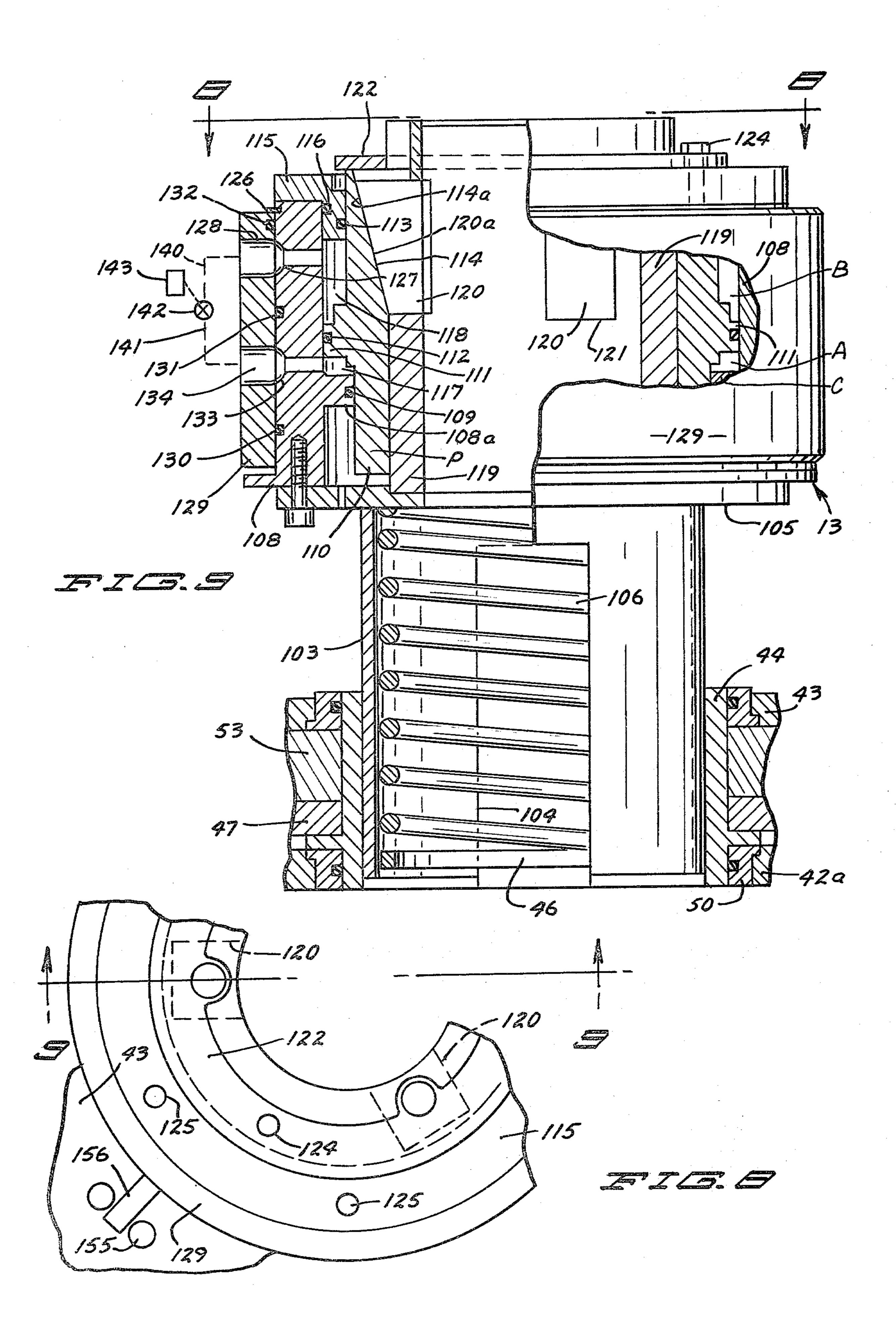
torque, high speed and thence at a high torque, low speed to threadingly couple a pair of rods.
