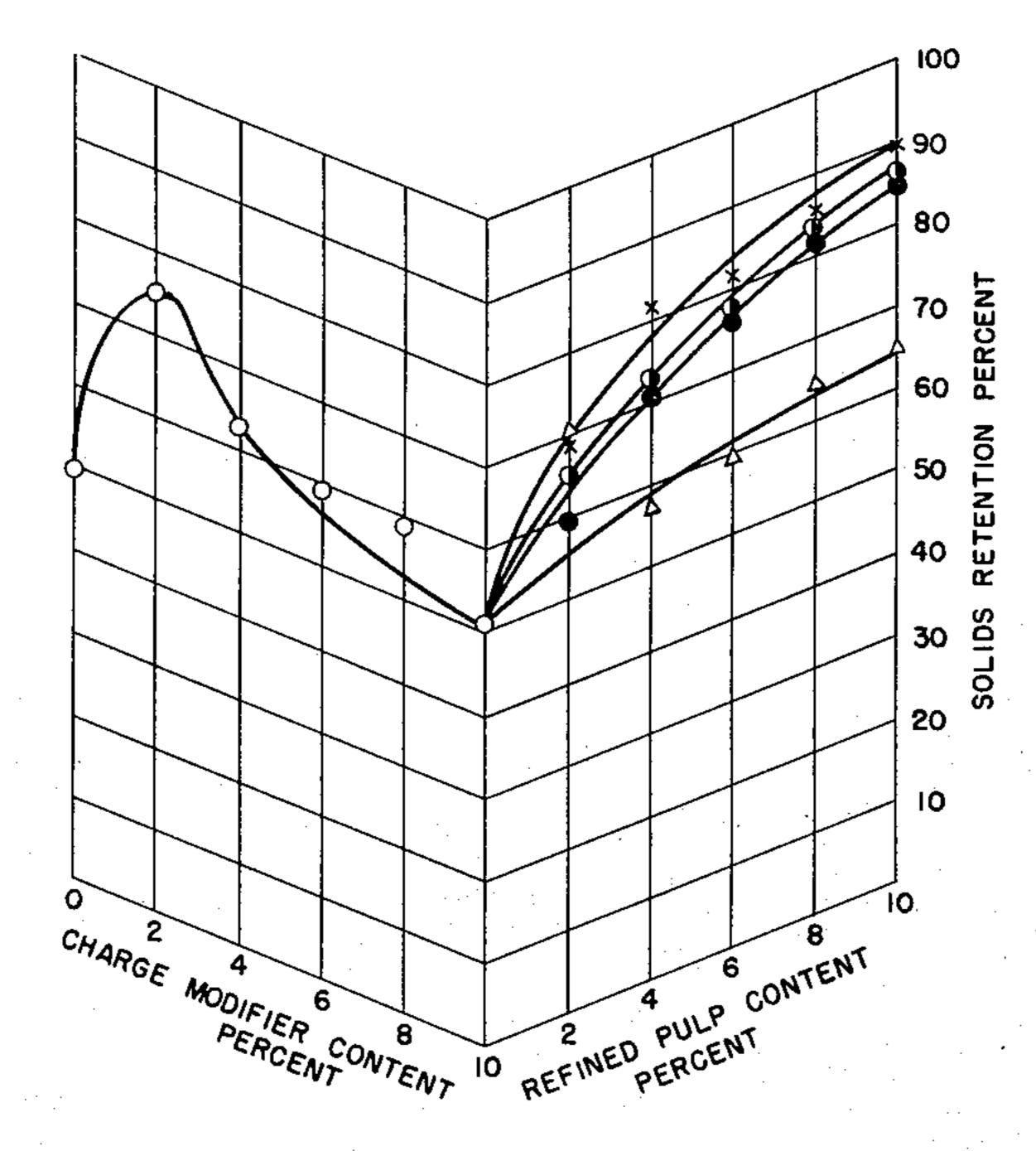
CHARGE MODIFIER: MELAMINE-FORMALDEHYDE CATIONIC COLLOID 70% PARTICULATE: DICALITE 215 DIATOMACEOUS EARTH 30% UNREFINED PULP/REFINED PULP REFINED PULP FREENESS, C. S. F. (INVERTED)
