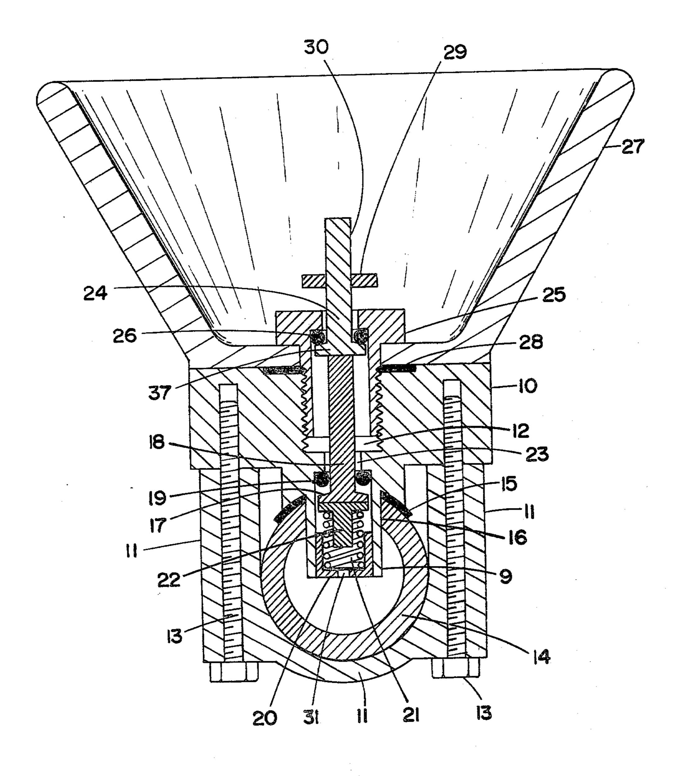
ployed to ensure a water tight seal between the water supply pipe 14 and the base member 10.
