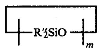
where R" can be the same or different monovalent organic radicals such as methyl or phenyl and m is an integer equal to 3 to 8 inclusive. An example of an organosilicon cyclic is hexamethyl trisiloxane, octamethyl tetrasiloxane, etc. The products made in accordance with the present invention are high molecular weight oils and gums.
