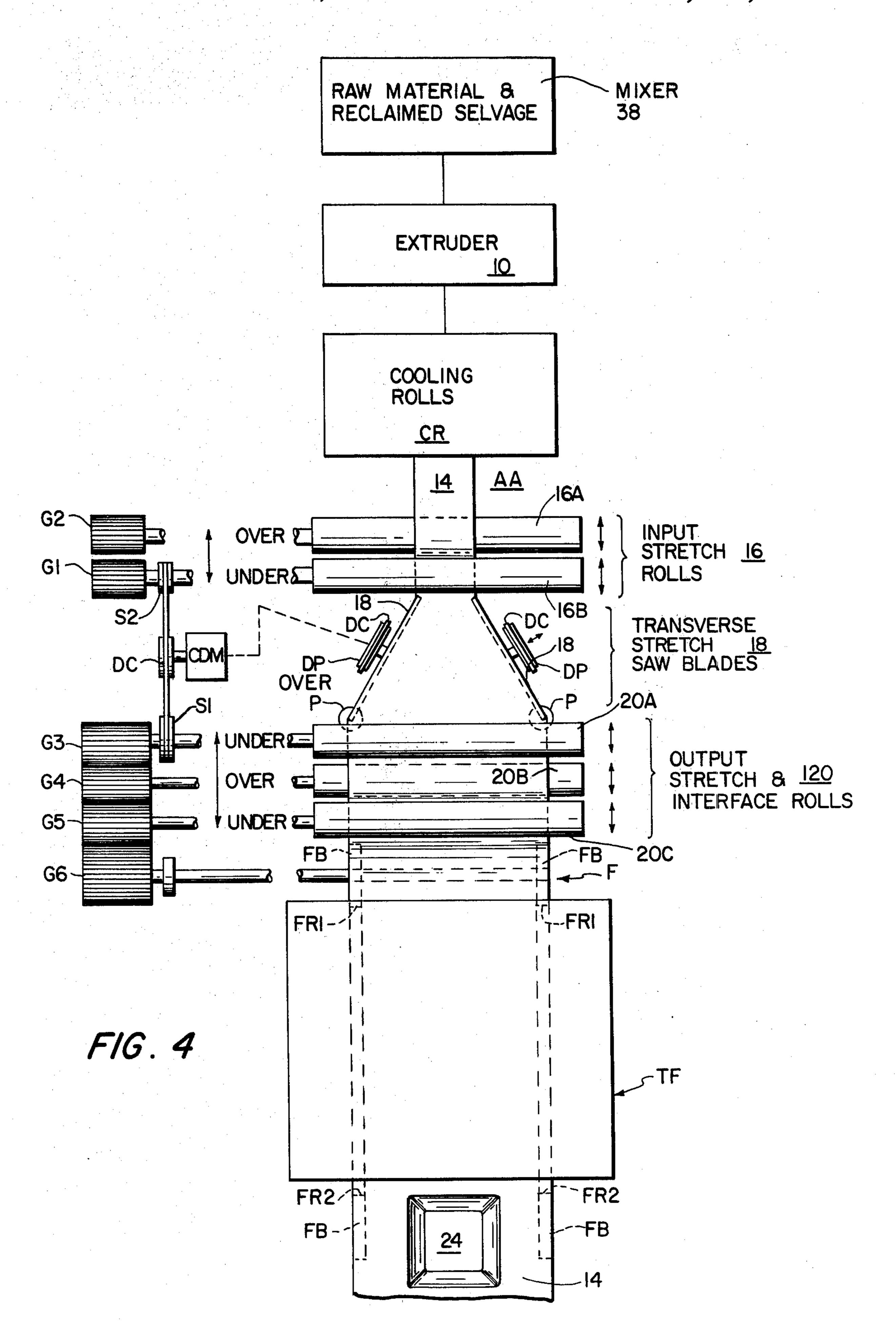
METHOD FOR THE CONTINUOUS FORMATION OF BIAXIALLY ORIENTED THERMOPLASTIC MATERIALS AND FORMING ARTICLES THEREFROM BY INTERMITTENT FORMING MEANS INTERFACED THEREWITH
