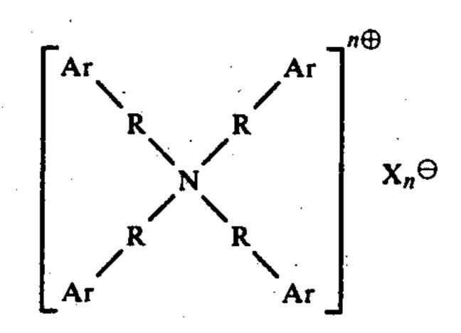
wherein each Ar is identical and is phenyl or a condensed polynuclear aryl group having 2 to 4 aryl nuclei,  $^{30}$  each R is identical and is alkyl of 1 to 4 carbon atoms,  $X\Theta$  is a salt-forming anion of valence 1 or 2 and n is 1 or 2 depending on the choice of X.
