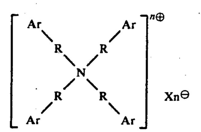
wherein each Ar is identical and is chosen from the group consisting of phenyl, naphthyl or phenanthryl, each R is identical and is chosen from the group consisting of ethyl and butyl and  $X\Theta$  is an anion chosen from the group consisting of chloride, bromide, iodide, and sulfate.
