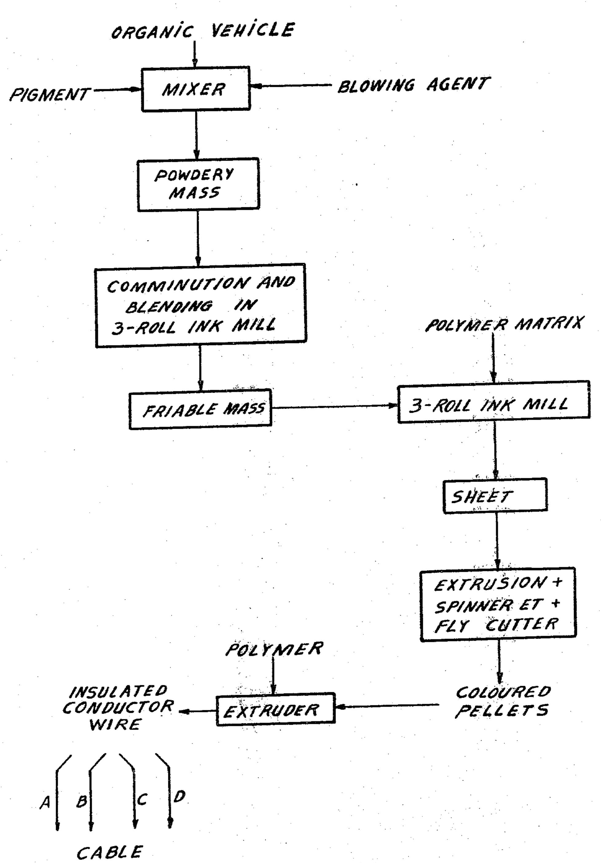
METHOD PRODUCING A COLOR CODED, CELLULAR THERMOPLASTIC RESIN COATED WIRE AND THE MATERIALS NECESSARY FOR THE COATING
