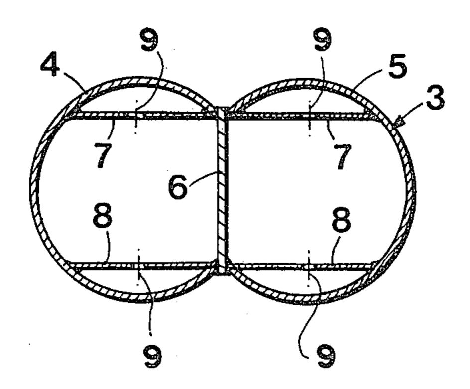
DRAFT TUBE FOR A REACTION TURBINE
