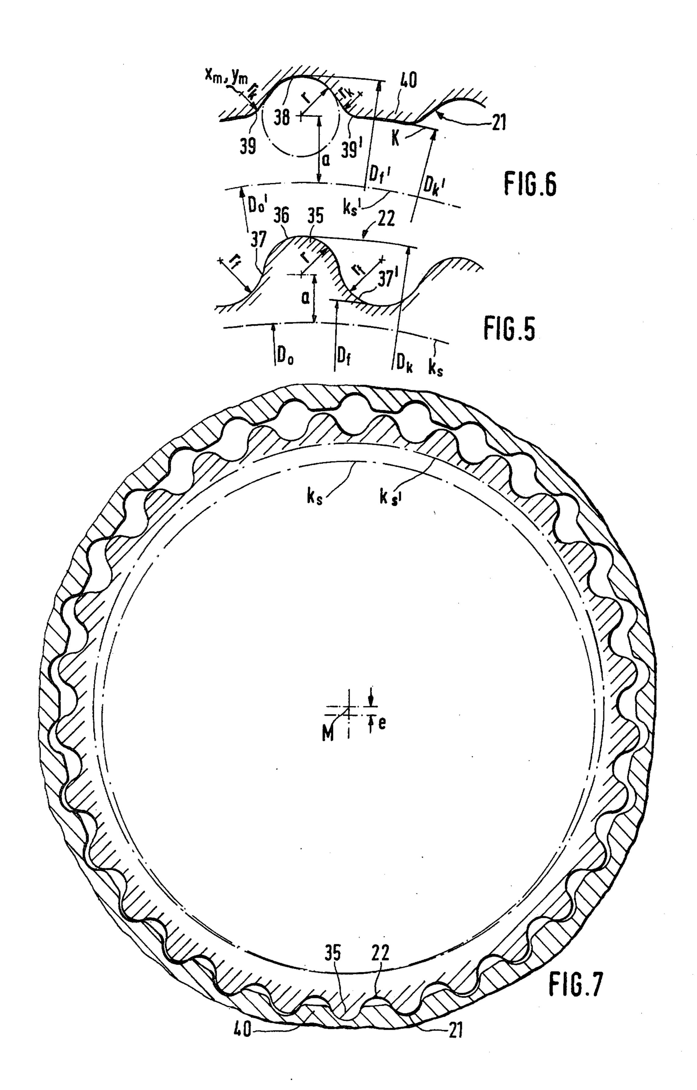
the one gear and transit into a tooth tip the outline of which substantially coincides with the crown circle, have a radius of curvature adjusted to the cycloid root line and the tooth tip section.
