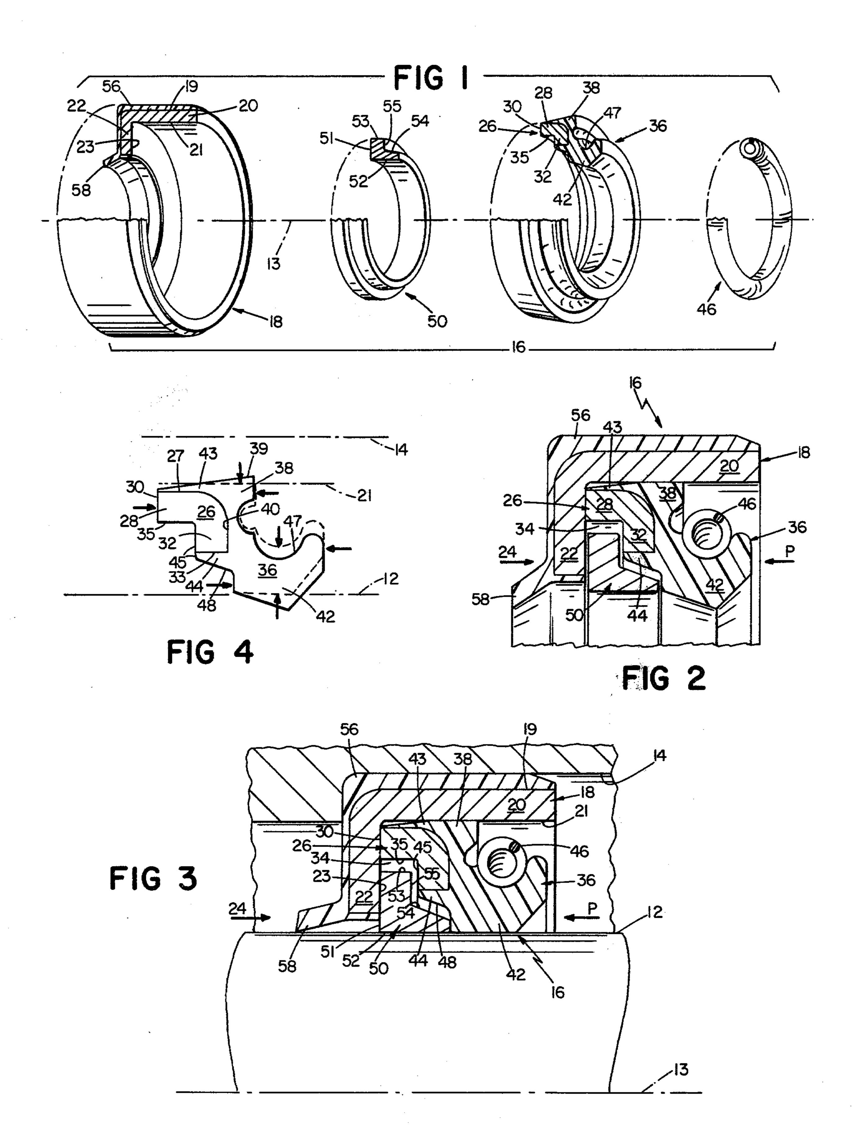
movement therein with its inner surface engaging the shaft.
