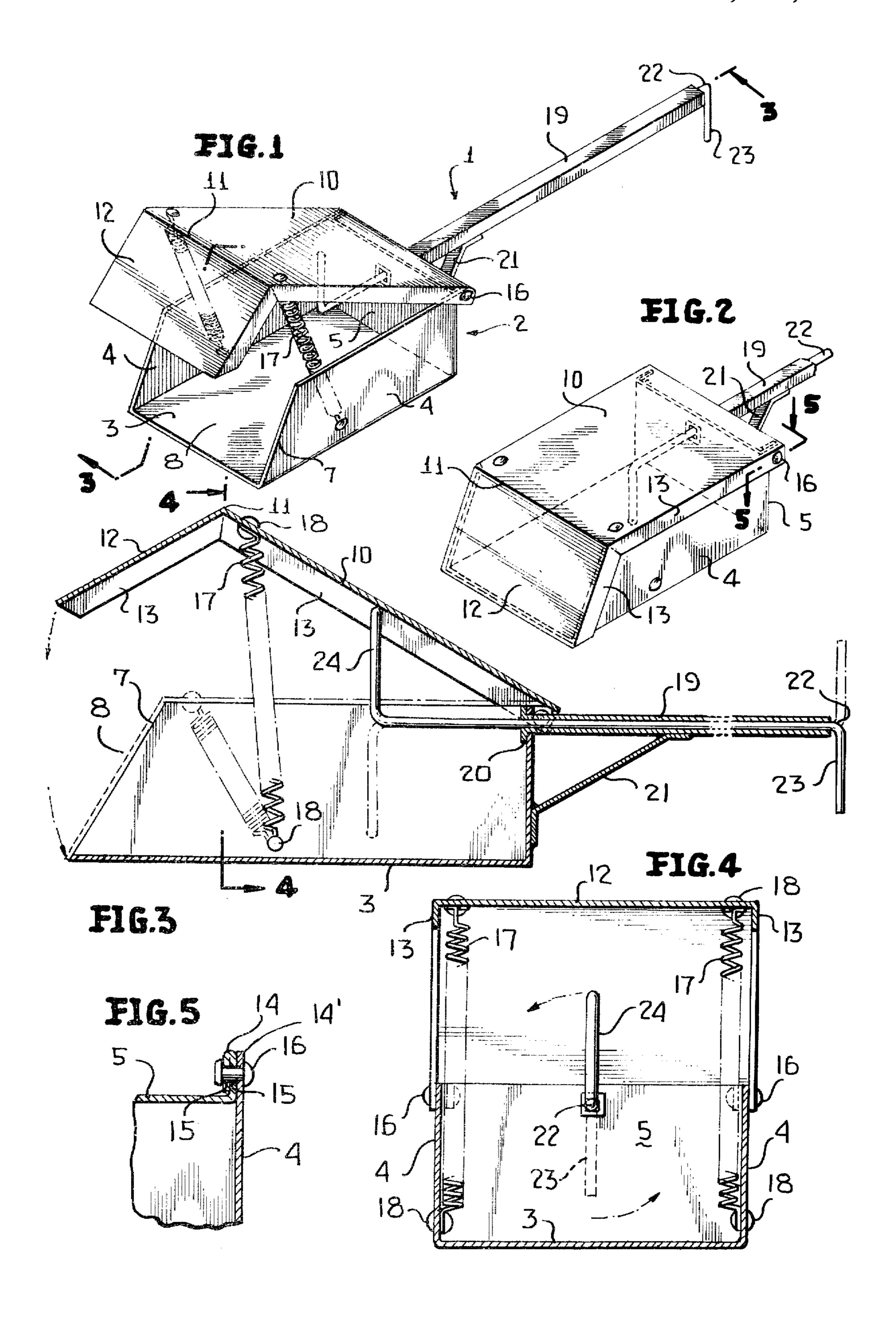
side walls slope upwardly and rearwardly, as at 7, to provide an open front end 8.
