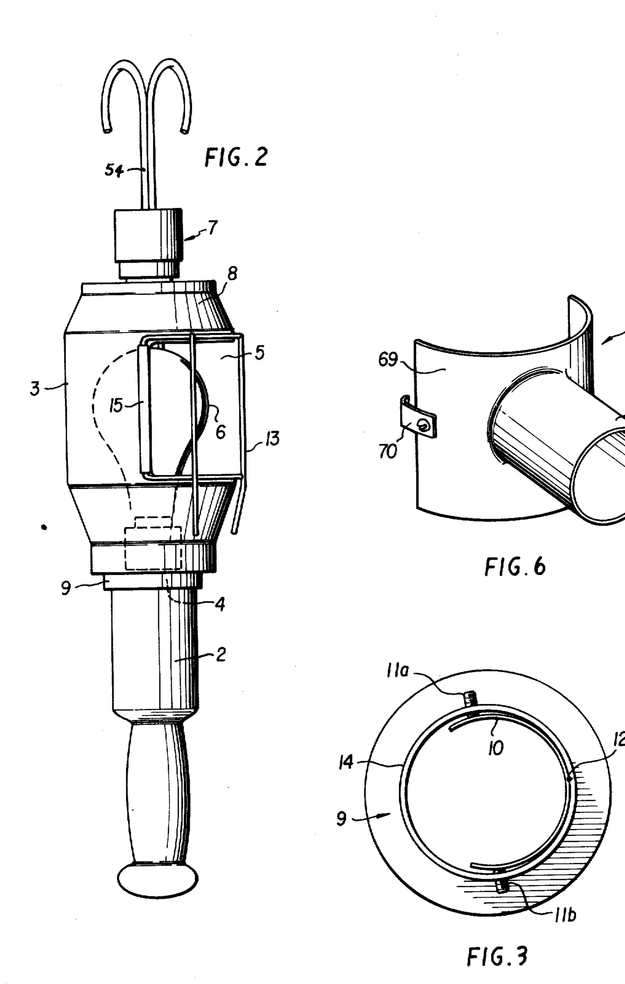
U.S. Pat. No. 3,808,420, which must be pulled away from the body of the light shield member before an angular adjustment may be made.
