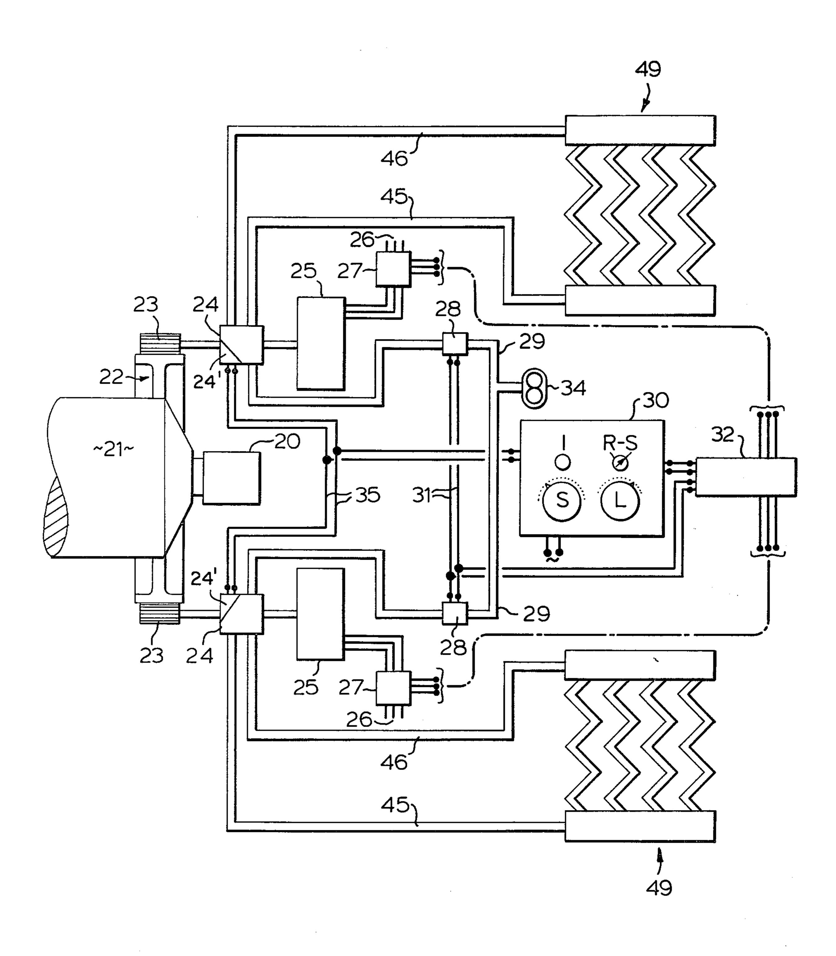
Alternatively, pulsed inching can be achieved by cyclically engaging and disengaging the clutch so as to provide a slow, pulsed forward motion.
