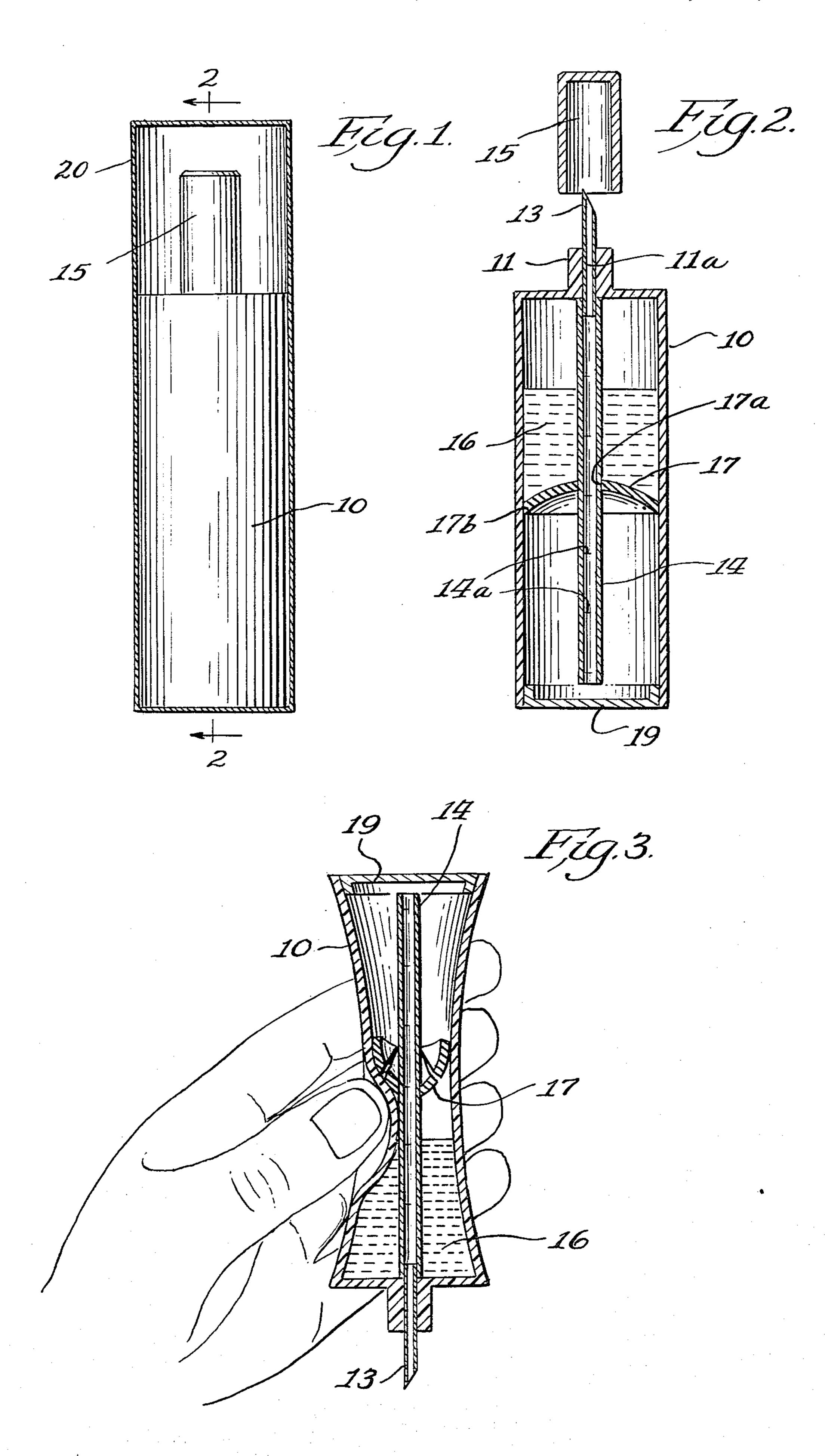
terminate short of the lower end of the container, as shown in FIG. 2. The tube 14 is marked with a series of graduations 14a. The container receives a cap 15 fitted with pressure on the neck 11 to protect the pointed end of the needle from injury or contamination.
