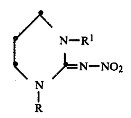
wherein R is hydrogen, alkyl of from one to six carbon atoms or alkanoyl of from one to seven carbon atoms, and R<sup>1</sup> is hydrogen or alkyl of from one to six carbon atoms, useful as insecticides.
