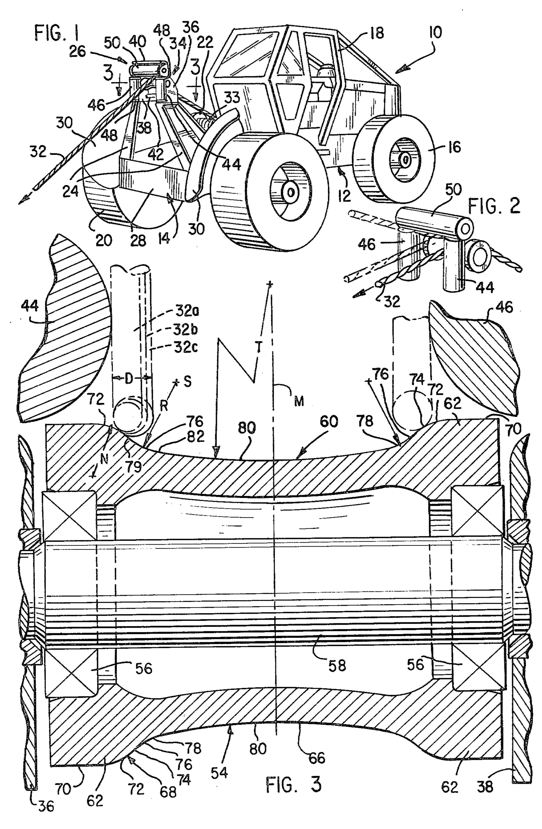
ing the cable into the center of the roller where it can run a groove therein after a period of use.
