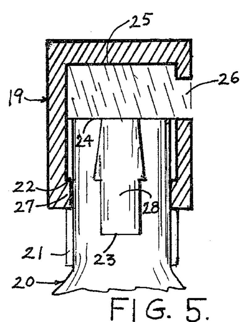
also be afixed to the container by means of a slide arrangement as shown in FIGS. 4 and 5.
